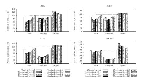
Fig. 4. Performance of checkpoint-based algorithm with different p values, normalized against the performance of the classical backfilling algorithm, which is marked by the dotted "100%" reference line. The "Classical, Actual" bar shows the performance with the classical algorithm, but supplied with the actual wall time (i.e., without any estimation error).
