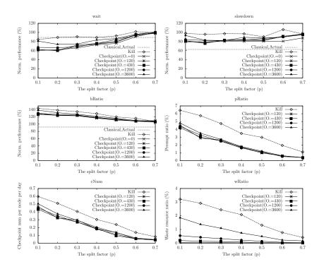
Fig. 7. Evaluation the impact of checkpoint overhead using ANL trace. Different checkpoint overhead are simulated. The simulate results that using classical backfill algorithm with runtime estimate are the baseline.
