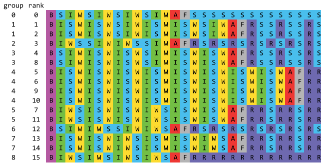
Fig. 12. Partial communication sequences for LU with 16 processes. (B=MPI_Bcast, S=MPI_Send, I=MPI_Recv, W=MPI_Wait, A=MPI_Allreduce, F=MPI_Barrier, R=MPI_Recv).
