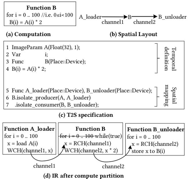
Fig. 1. An illustration of the T2S approach.
