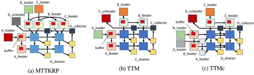
Fig. 8. Systolic arrays for the FPGA workloads.
