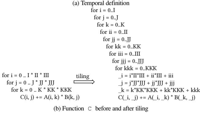
Fig. 2. Temporal definition of matrix multiply, including tiling.
