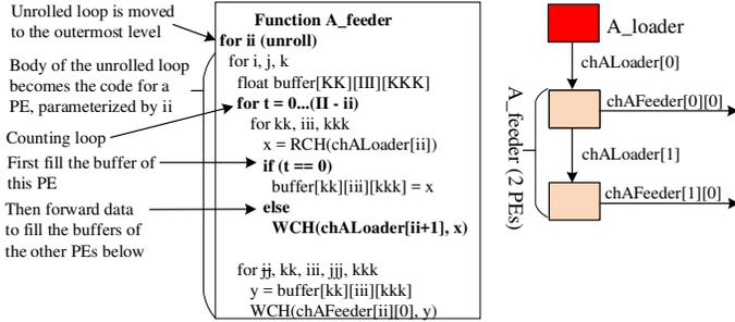
Fig. 5. IR of `A_feeder` after loop unrolling and data scattering in Fig. 3(e). The resulting changes to `A_feeder` relative to the IR in Fig. 4 are highlighted in bold fonts. The changes to `A_loader` (not shown) are that due to loop unrolling, channel `chALoader` is split into an array of channels `chALoader[0..II]`, and then due to data scattering, this array of channels are scattered across the `A_feeder` PEs as shown in the right of the figure, and `A_loader` writes only to `chALoader[0]`.
