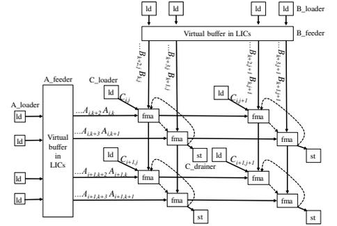
Fig. 9. Systolic array for GEMM on the CGRA
